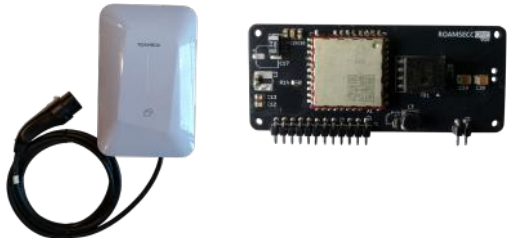
Pluggable charger-to-vehicle communication module
