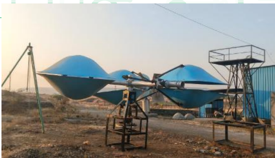
5 kW Vertical Axis Breezemill
