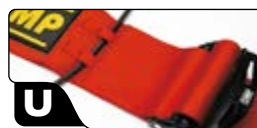
FIXING INTERCOM CONNECTOR
