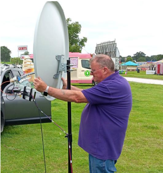
Fig.6 Alignment of the Dish with Data from Dishpointer
