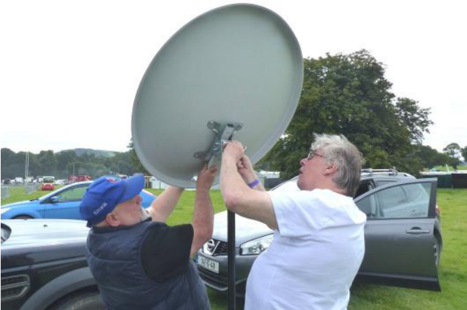
Fig. 2 Assembling and mounting the Dish on the Tripod
