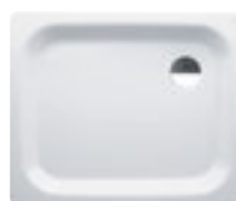
PLATINA Shower tray, rectangular, enamelled steel (3.5 mm), flat (65 mm) 900 x 750 x 30 mm
