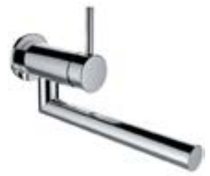
Concealed single lever basin mixer for Simibox 1-Point, swivel spout, projection 225 mm
