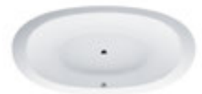
ILBAGNOALESSI ONE Bathtub, oval, drop-in version, with centre outlet, with frame, sanitary acrylic 2030 x 1020 x 460 (575) mm
