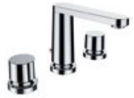
3-hole basin mixer, projection 130 mm, fixed spout, with / without pop-up waste lever, with pop-up waste
