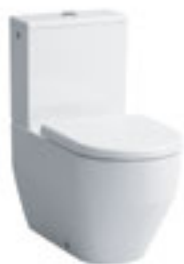
Floorstanding WC close-coupled, optimized for 4.5/3L / 6/3L, washdown, rimless, outlet horizontal or vertical 700 x 360 x 430 mm
