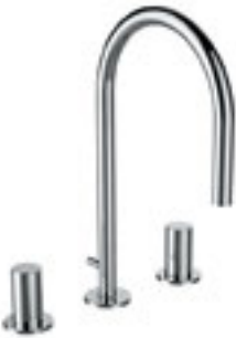
3-hole basin mixer, projection 166 mm, swivel spout, with pop-up waste lever, with pop-up waste / without pop-up waste valve
