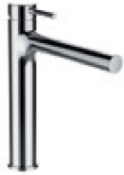
Column single lever basin mixer, projection 180 mm, height at perlator 190 mm, fixed spout, without pop-up waste
