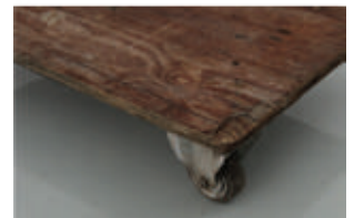
Wood: Splinters and rot.
