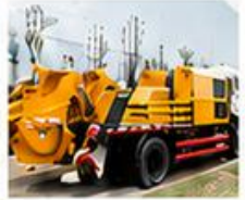
• Truck-mounted concrete pump
