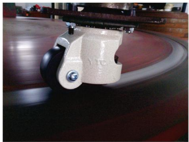
60 Adjustable caster load-bearing walk test at 300Kg
