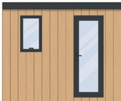
UPVC single door fully glazed left opening 600m wide by 1m high casement window
