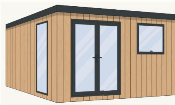
1.8m French doors 1.2m wide by 1m high casement window 600mm wide full length left picture window
