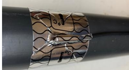
Fig 4 – Temperature Probe Installation
