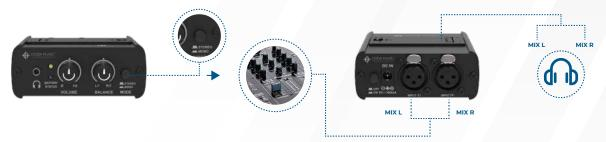
Depress the mode button for stereo selection on your IEM system. Connect two XLR cables between your IEM system and the mixbus or auxiliary of your sound board. This will send the Left and Right input signals to their corresponding headphone output channels. In Stereo Mode the pan control will adjust the stereo balance.
