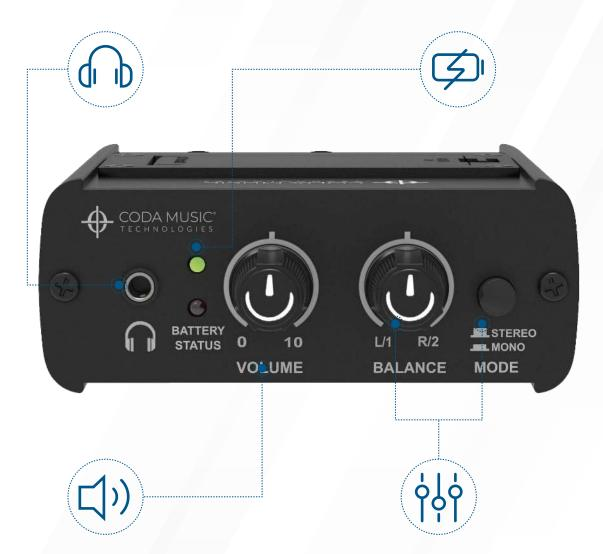
CLEARLY HEAR YOUR MIX -Enough power and control toclearly hear your mix overstage volume, even overdrums. PERSONALIZE YOUR MIX - Personalize your mix with both mono and stereo settings. In Stereo Mode the pan knob adjusts the balance between the left and right channels. In Mono-Mix Mode the pan knob adjusts the volume ratio between the left and right channels.
