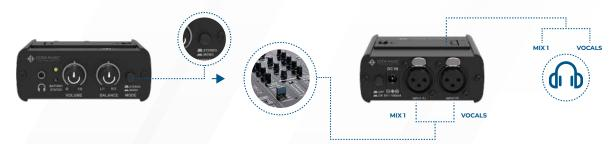
Mono Mode can also be used as an easy way to create a custom monitor mix such as having the band in one channel and your instrument in another. To setup Mono-Mix Mode, press the mode button down, for mono mode selection. Then connect the mix of the band to the left input on your IEM-STEREO and connect the direct output of your channel/instrument to the right. Now the pan control will attenuate the level of either the band mix or your own channel by moving it to the right or left.
