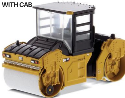
CAT CB-13 TANDEM VIBRATORY ROLLER WITH CAB
