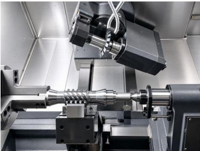
Worm Shaft being machined on WM 40100
