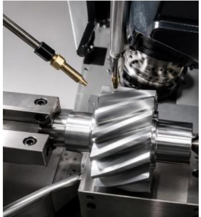
Helical Gear being gashed on WM 40100
