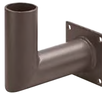
Flat Base L Connector Can be mounted on wall or flat surface on poles. Creates a 90 Degree Angle for Lights to be mounted with standard 2 3/8" Round Slip-Fit Head
