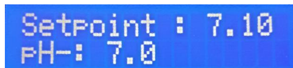
Figure 6 – Main Menu without Active Alarms
