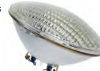
RP56S012300WF | BAI Reflector PAR56/WFL 12V 300W 4500lm 3000K 37° 113x178mm Especial Piscina
