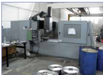
CASTOR LATHE Max. Diameter 1200 mm. Max. Length 4000 mm.
