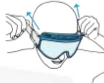
Pic.2 - Set the length of the elastic band by gently pulling back the ends.
