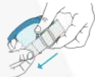
Pic.4 - Set the adjustment by letting slide back the loose end
