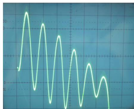
Fig. 4 Oscilloscope display of Frank-Hertz Experiment
