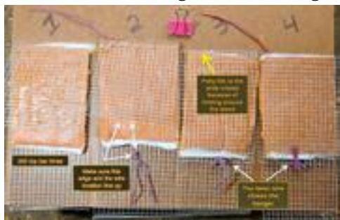
Figure 8 Loading a new hanger with a patty in four positions. See the thin red and blue wire about three inches long (position 1) to close the hanger. Locate that closing wire where it will close the end of the folded wire grid as shown in position 2. Fold over the closing wire on the long side of the hanger grid. With a patty loaded in the hanger, press the two wire grids together gently. Hook the closing wire tails through to the opposite grid as shown in position 3. Thread the closing wire tails back through to the other grid and make a snug closure from the other side of the hanger, as shown in position 4. The small pink binding clip at the top of the figure can close the grids too. I cut the one-pound patties approximately into thirds with a box cutter or a large pizza cutter.
