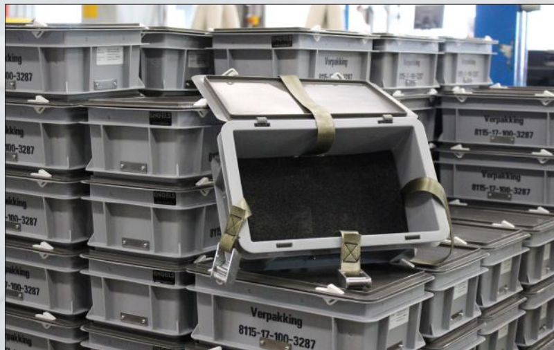
Straps and foam instead of shock absorbing filling material.
