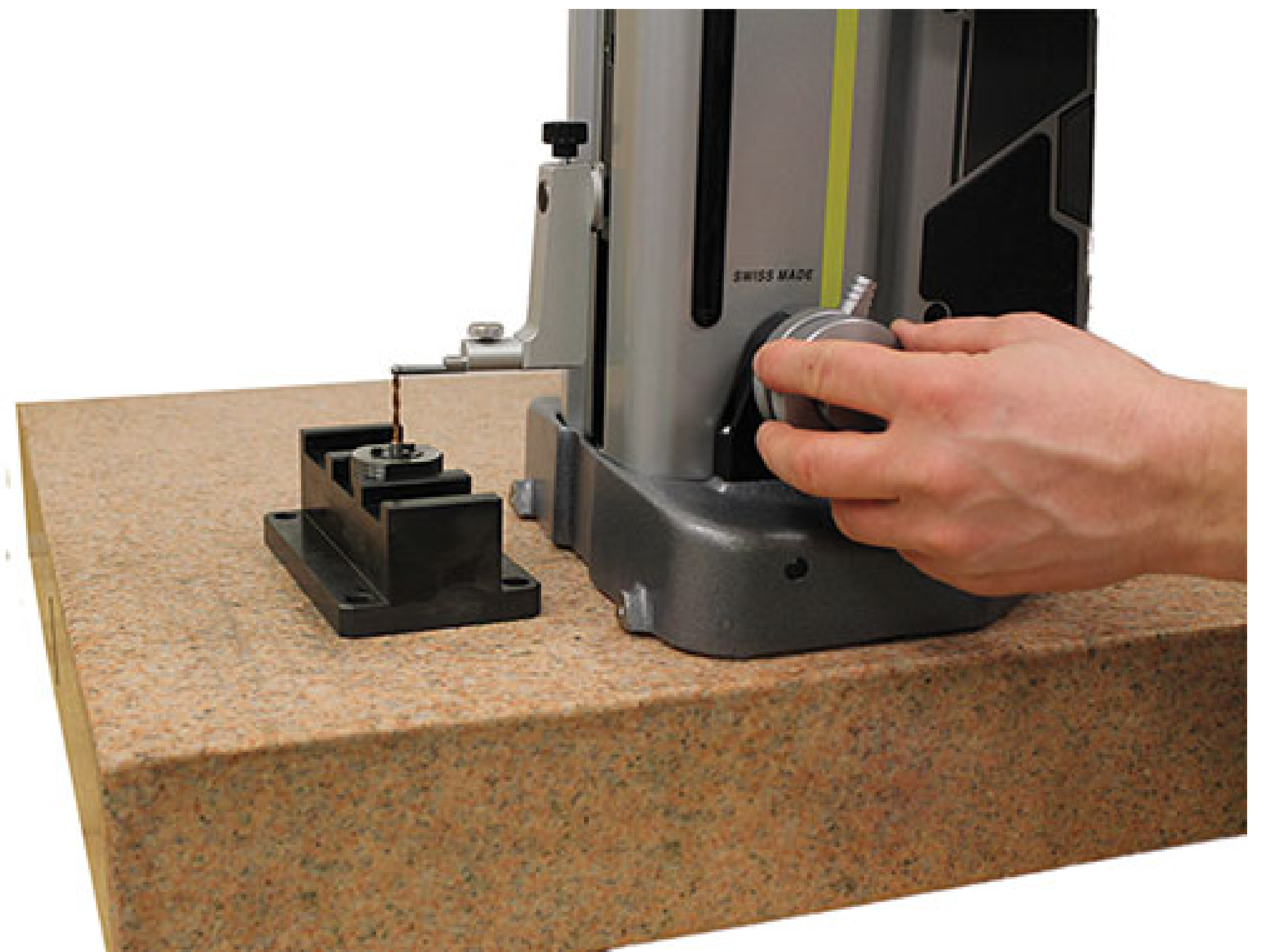
Offline measurement of cutting tools does not require any special equipment, as shown in this example using a presetting block from National Machine Products. (Provided by Tsugami/REM Sales)
