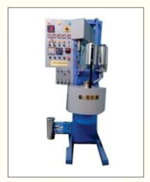
**Bottom Pouring Type Stir Casting Setup**
