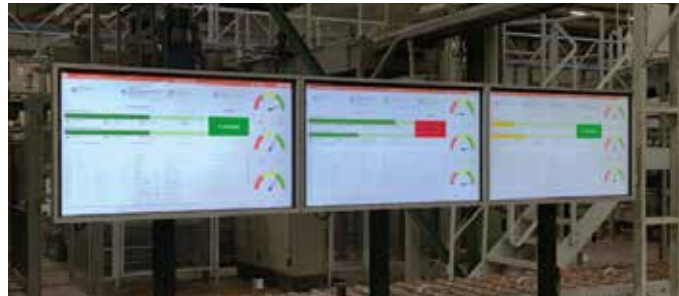
Visual Factory: Actual performance is displayed in real time on large screens in the production halls. (Source: Sika)
