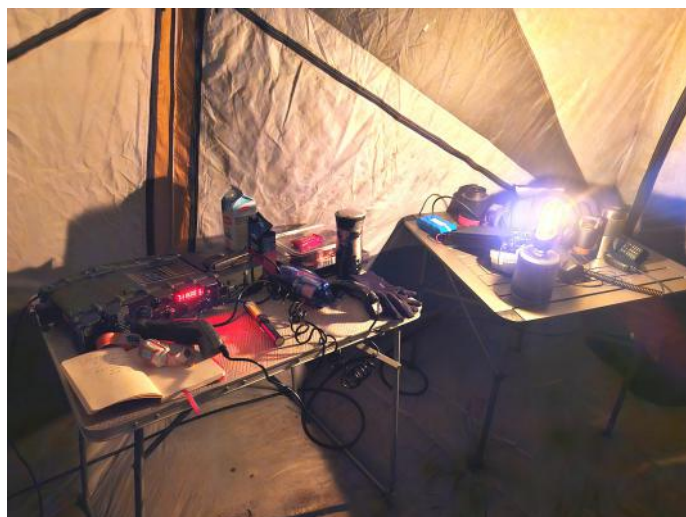
2: The two operating stations: PRC-320 on the left and Xiegu G90 on the right.
