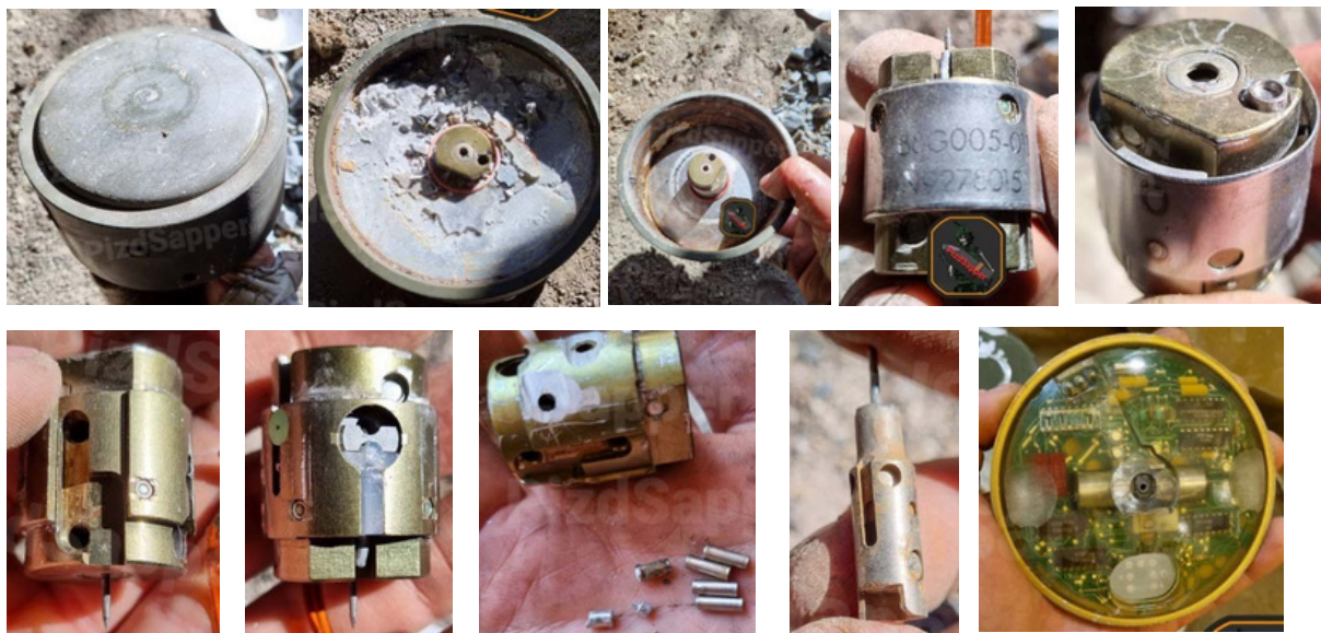
General internal structure of the M70 mine
