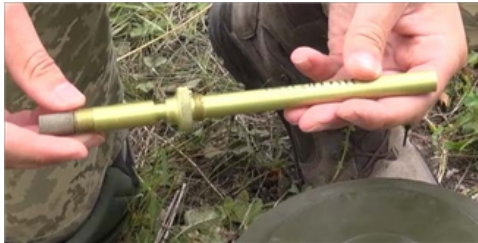
Pin-type target sensor sleeve
