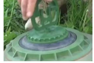
Setting the detonator to the live position
