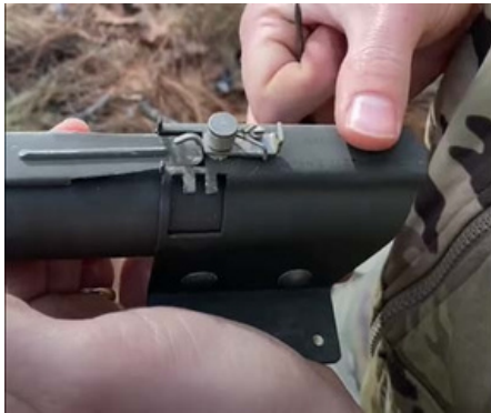
Install the mine and the target sensor. The sensor is secured in the "eye" of the lever
