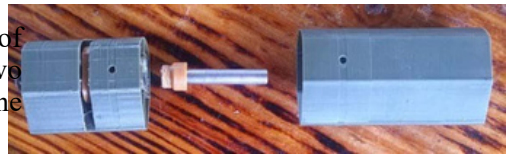
Left: a disassembled mine; the pin holds the striker in place. Center: the bottom of the “cup” where the explosive charge is packed. Right: Cap with an MD-5M detonator
