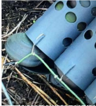
A makeshift cassette system for dropping “PRYANIK” mines from a drone. Visible are perforated tubes—blue in color—and lids, as well as some sort of rubber band involved in the system for holding the lids in place and then opening and releasing them.
