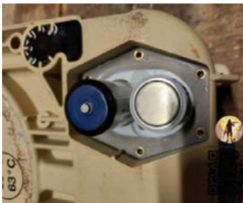
Compartment containing two lithium-ion batteries.
