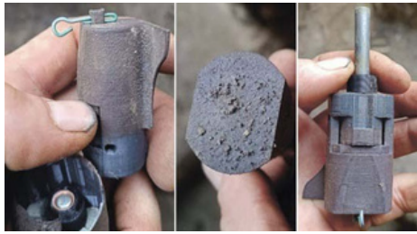
Left: a disassembled mine; the pin holds the striker in place. Center: the bottom of the “cup” where the explosive charge is packed. Right: Cap with an MD-5M detonator
