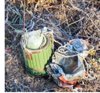
The DM1399 mine has deployed correctly. The parachute and sensor antenna are visible. The target is sticking out.
