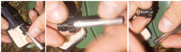
3D sleeve with a primer fitted onto KD No. 8A
