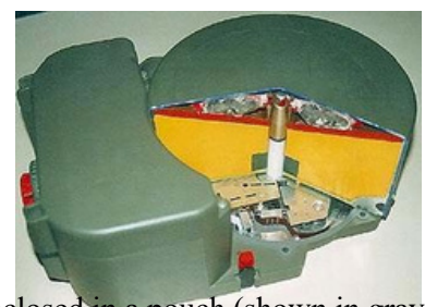
Compartment containing two lithium-ion batteries.
