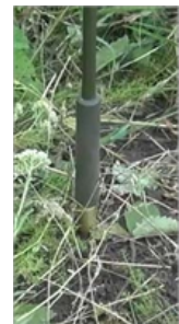
Avoiding tilt, install pin sensor
