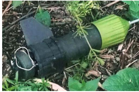
Debris from a POM-S mine. The self-destruction unit is visible. The casing has shifted. The target sensors did not deploy.
