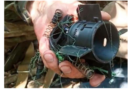
The mine landed flat. The tail section themselves: Threads, springs, weights. The tail section
