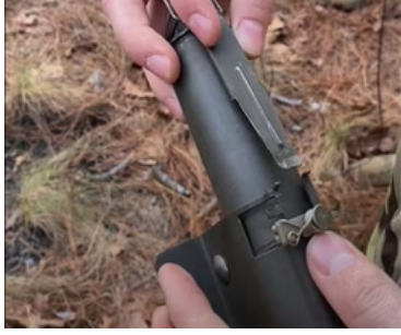
Loosen the screws and remove the mine the housing place
